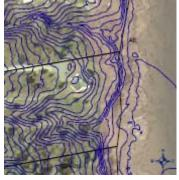
County. LIDAR, standing for Light Detection and Ranging produces detailed topographic information
