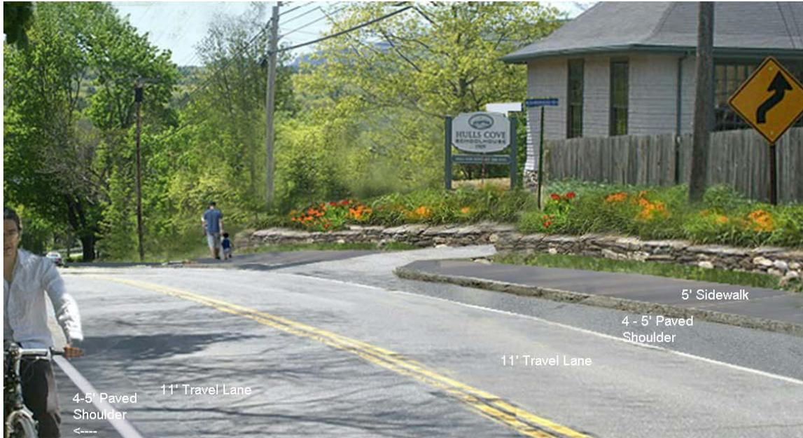
**Figure 4 Conceptual Illustration of Sidewalk and Shoulders**
