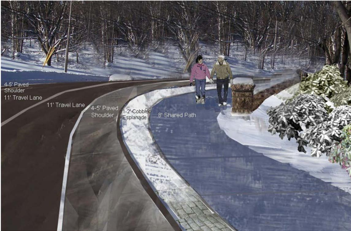
**Figure 8 Conceptual Illustration of Route 3 Curve Near Harbor Lane**
